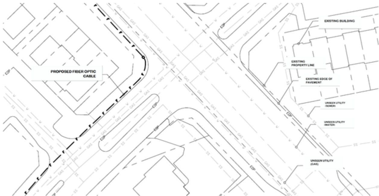
Figure B-1. Sample Plan Sheet with Suitable Line Weights and Annotation. Note: Annotations for travel lanes, road names, numbers, clear zone, and ROW were omitted for clarity.
